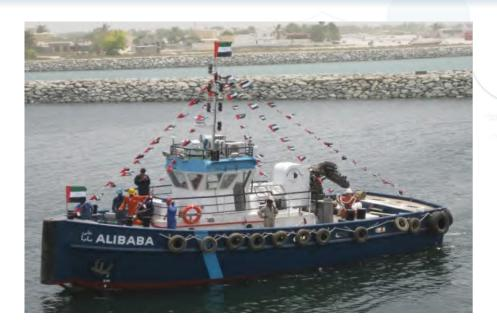
Registration Dimension 17.15 meters Year Built Length Overall 2010 Port of Registry Length B.P. 15.48 meters Dubai-UAE Breadth 5.31 meters Official Number 6444 Depth 3.06 meters Classification **RINA** Draft 2.20 meters Flag U.A.E.
